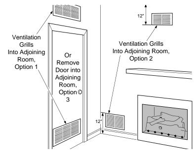
Figure 3 - Ventilation Air from Inside Building
